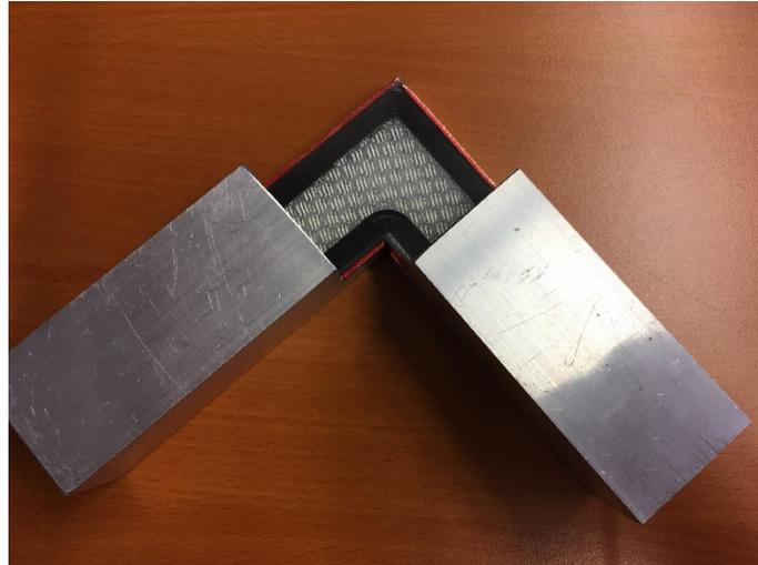
L-profile in housing. Housing protects laminate from impacts.
