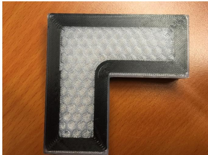
Concentric orientation of the reinforced fibers allows a derivative of the forces.
