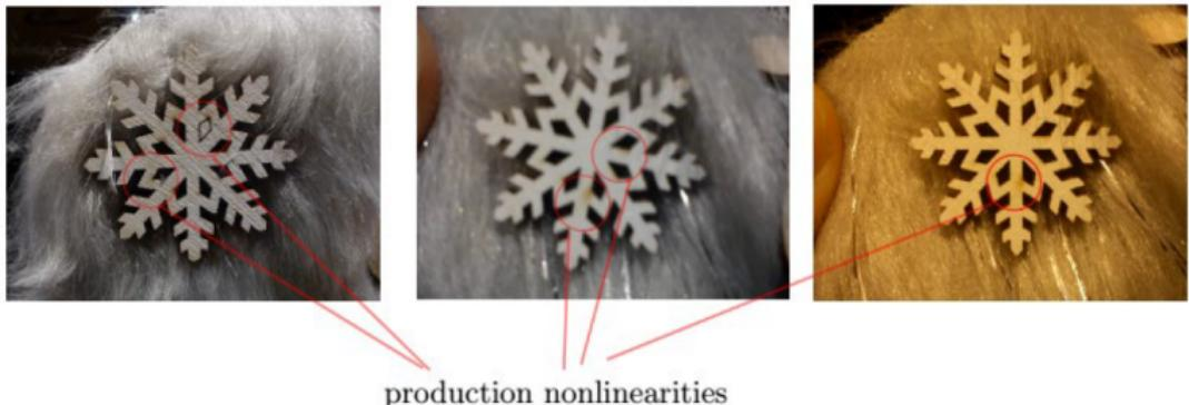
Figure 1: Non-linear production phenomena in lasercutting
