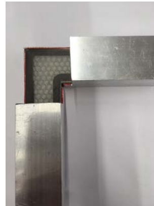
Fig. 9: Application concept of 3D-printed fibers for the reinforcement of edges in the MMO3D project
