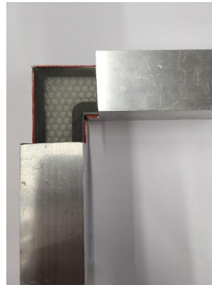
Fig. 14: Application concept of 3D-printed fibers for the reinforcement of edges in the MMO3D project
